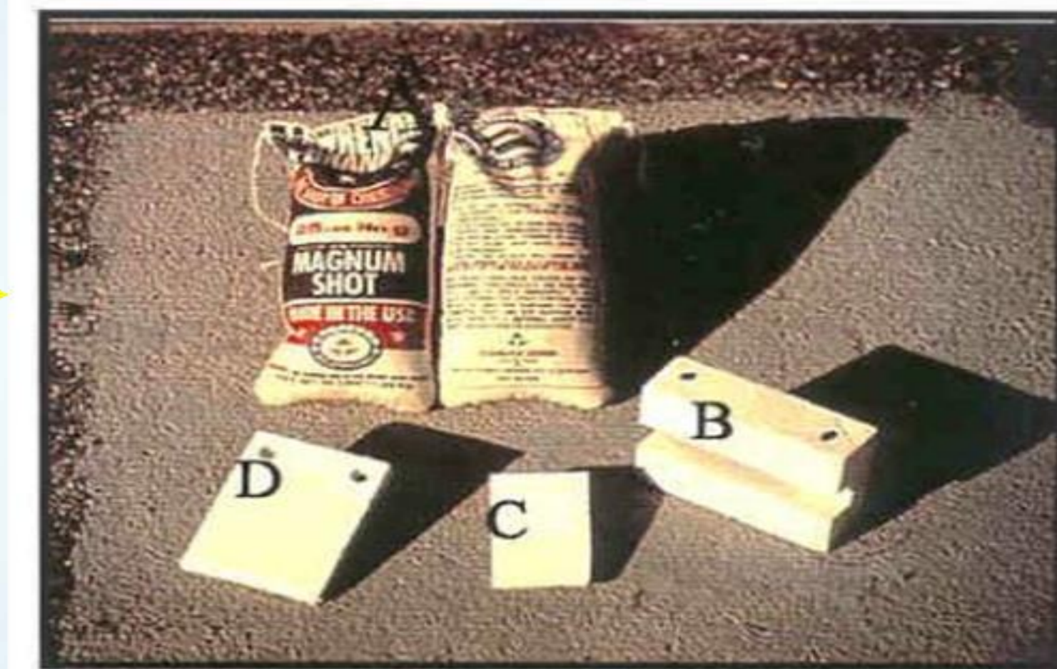
Clockwise from Top Shielding: A. #9 Lead Shot - 25 lbs. each B. Tunnel Lead Brick C. Small HVL D. Remote Use Two HVL
